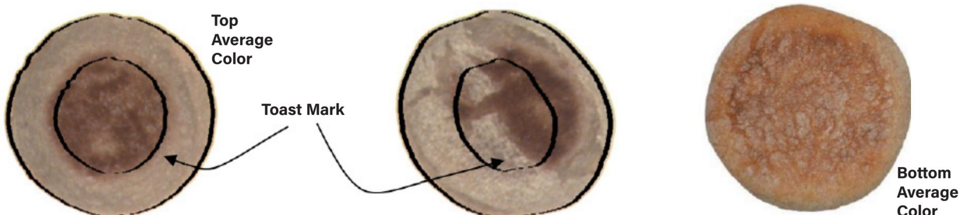
**True color calculations**, on both the top and bottom surface of the product, are measured in various units such as  $L^*a^*b^*$  and BCU. The top toast mark may be quantified specifically for size, location, and color, with respect to the whole surface or the central region alone.
