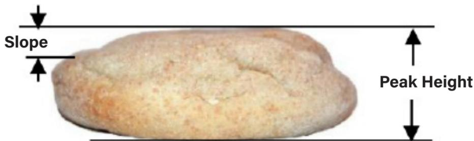
**Profile height calculations** are based on hundreds of individual height values gathered on every product, which leads to a measurement accuracy of  $\pm 0.5\text{mm}$ . **Mean Height** is another common measurement applied to english muffins.
